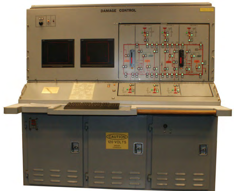
Figure 6-31 — Damage control console.
