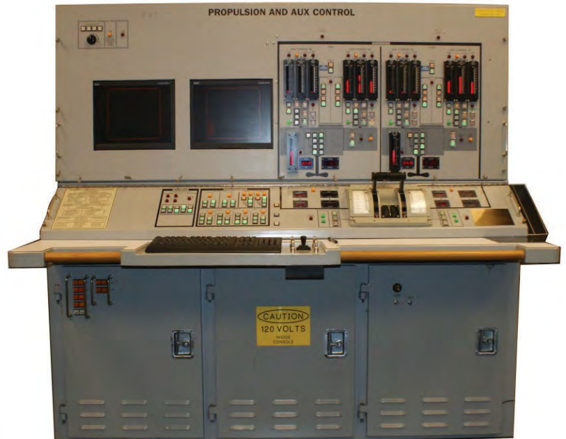
Figure 6-27 — Propulsion control system.
